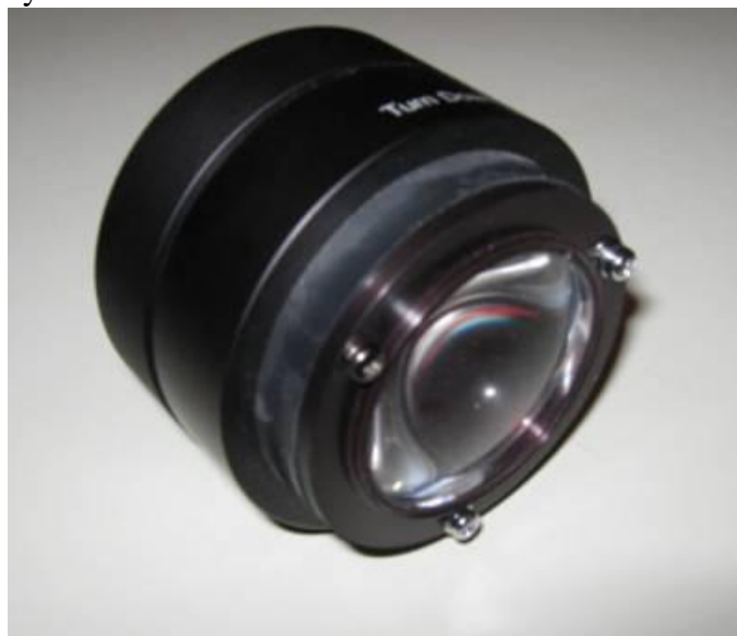
Collector lens assembly after removal from the lamphouse. The lens surface at the lower right faces the bulb. The flange at the upper left mounts to the microscope.
