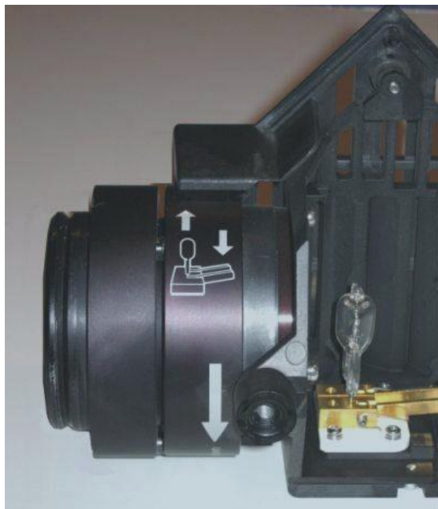
Lamphouse with cover removed. 12 V 100 W bulb is on the right and collector lens assembly is on the left.
